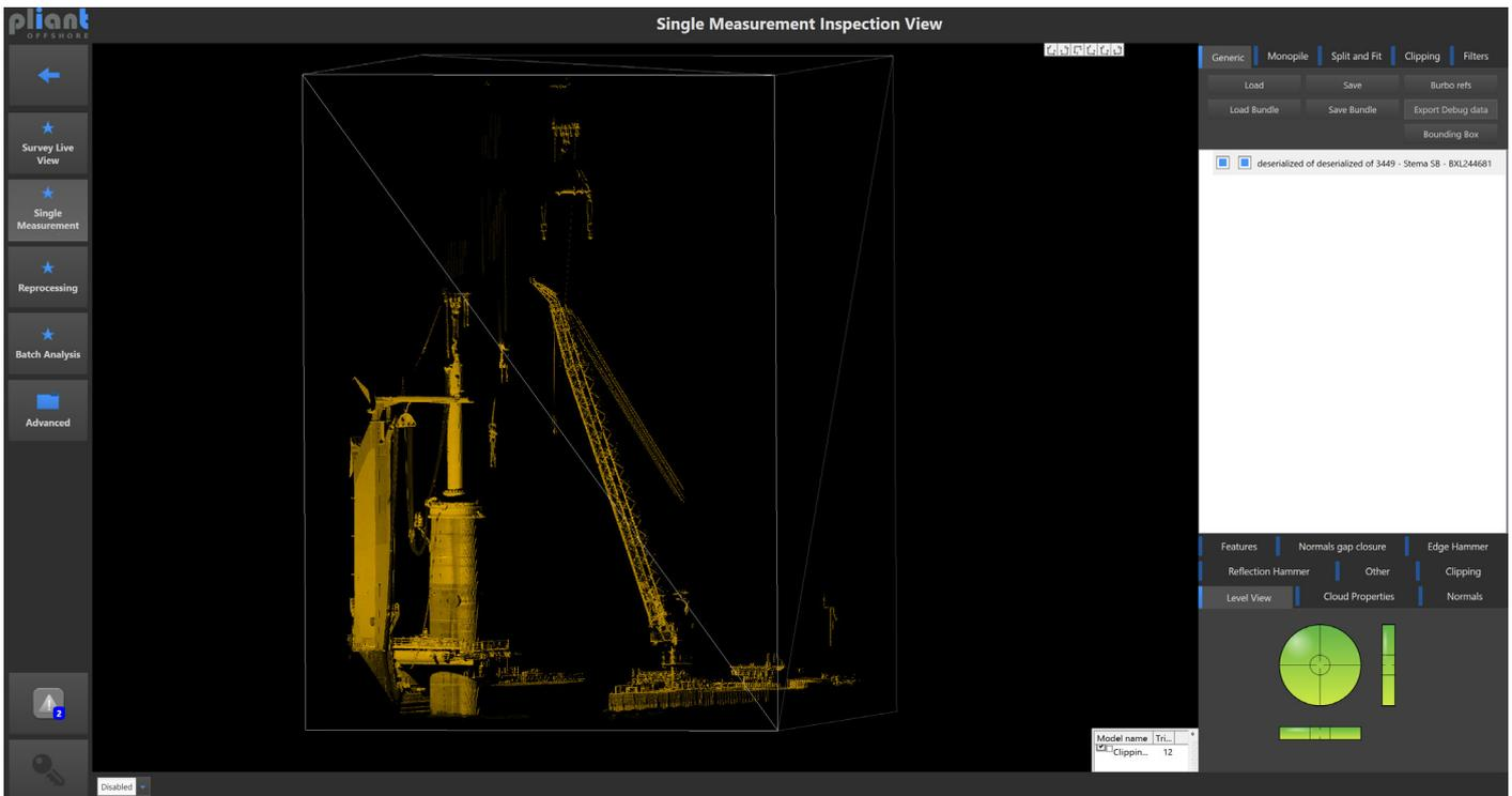
In addition, production faults or irregularities do not present a direct risk of misplacement. The complete three-dimensional image compensates for small deviations. And because all measurement data are stored, you can provide evidence in case of a conflict about a deviating monopile position afterwards.”
